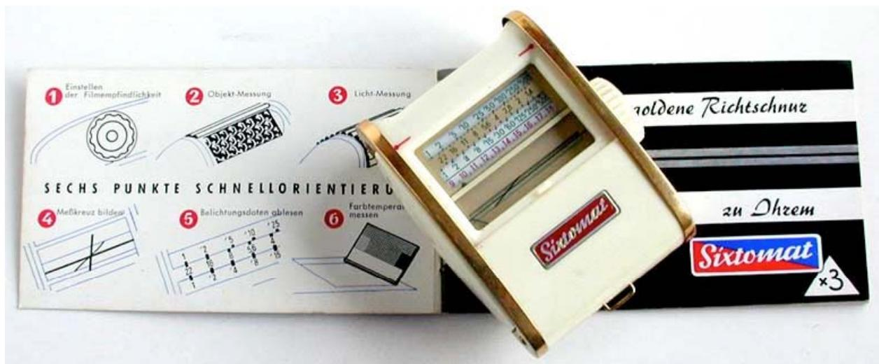
This *Sixtomat*<sup>15</sup> was manufactured by Gossen from 1952 to 1958. The case is of an *ivory-look* plastic and the trim is of brass. A roller-blind doubles as cover and as incident light<sup>16</sup> hood. The *Sixtomat* is calibrated for both the German DIN and the American ASA systems for rating film speed. Although perhaps more attractive than most, this meter was fairly representative of those made in its day.
