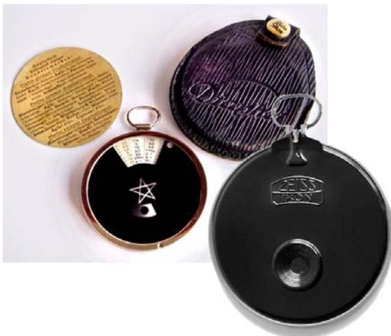
back and rotated the wheel within so that you viewed the subject through a graded series of filters. The last in which the subject was visible was converted to your exposure on the front of the *Diaphot*.
